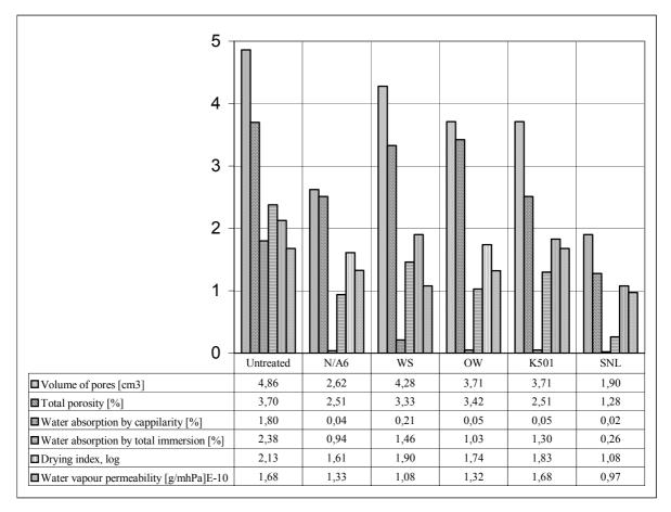
Figure 2. Porosity and hygric properties of the water repent products on travertine.
