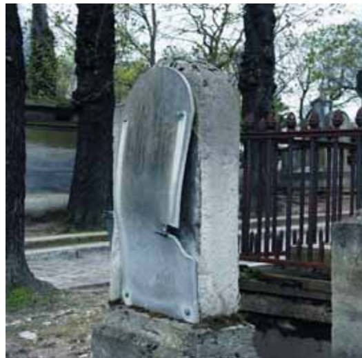
Figure 2: Bowing phenomenon observed on old gravestones, Paris
