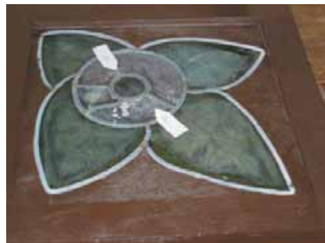
after 2 months in 40% acetic acid at RT and 4 h boiling
