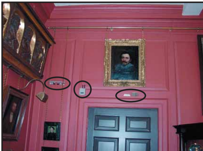
Figure 1: Microclimate monitoring in English Heritage Ranger's House, Red Evocation room (Wernher collection). Data loggers from left show pollutant samplers, RH and T and MIMIC PQC passive box and palette
