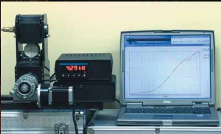
Fig. 1: Complete portable testing setup during split tests. The testing device equipped with stepper engine is operated by laptop with software for data acquisition and analysis. An accessory gear-box is inserted between the stepper engine and the loading screw in this case. Loading displacement data are obtained non-directly by counting the loading screw revolutions. The maximal displacement velocity is 1 mm/min in the case of the stepper engine in use.
