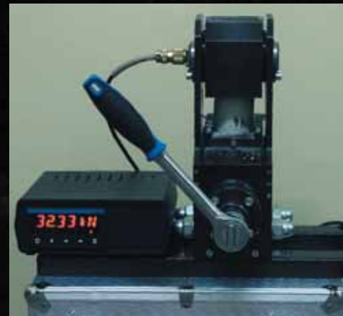
Fig. 2: Portable testing device with manual loading during compression tests. Screw rotation is carried out manually using a ratchet wrench. Only the maximal loading force is measured using this layout.
